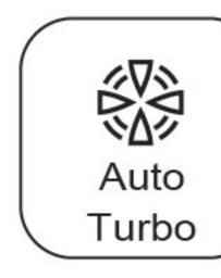
Tap 🐯, the smoke baffle shield will be on automatically, and the impeller will run at the Auto state; tap 🕸 again, the impeller will stop.
