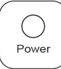
Tap  $\bigcirc$ , enter the standby state, and then operate other buttons. (The device will automatically shut down if no operation on other buttons in 2 minutes) When the impeller is in the operating state, tap  $\bigcirc$ ,  $\bigcirc$  will flash, and the impeller will enter the delay state and then shut down automatically after 2 minutes; tap  $\bigcirc$  again, the impeller will shut down directly.
